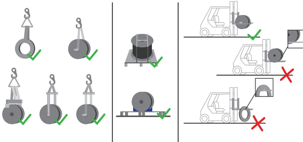
Figure 28 Rope handling recommendations
