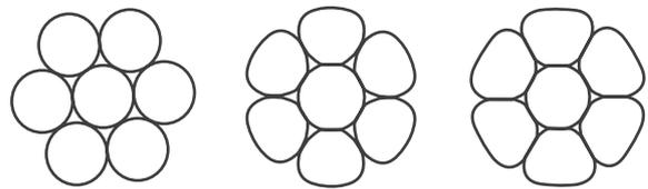
Figure 10 Round strand, light and high compacting level
