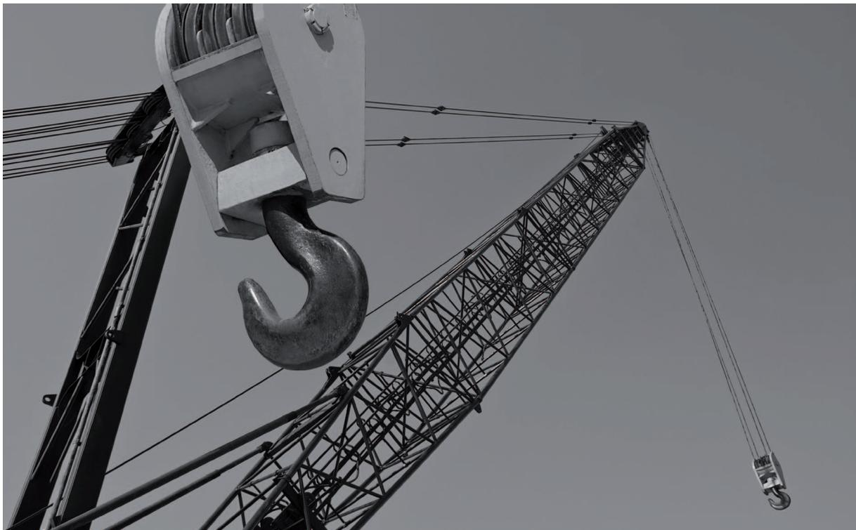
Figure 22 Multiple fall lifting
