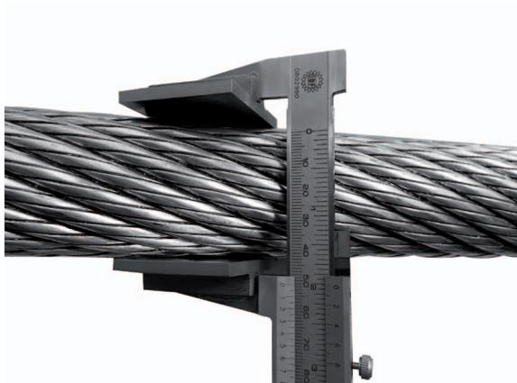
Figure 1 Diameter measurement
