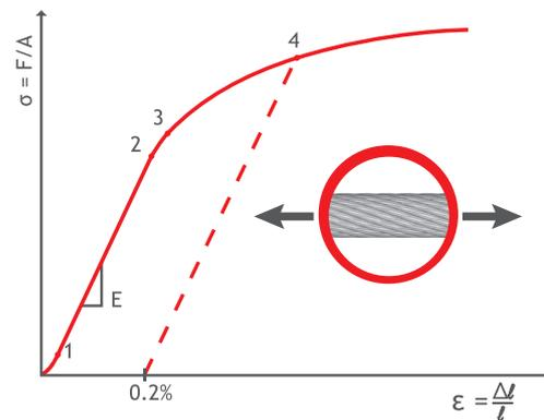
Figure 17 Stress - strain curve for a wire rope
