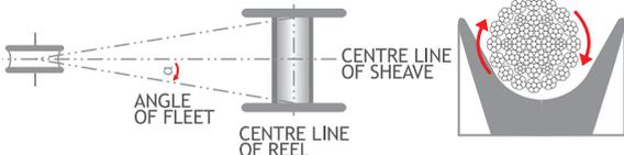
Figure 13 Fleet angle during spooling and rope rolling
