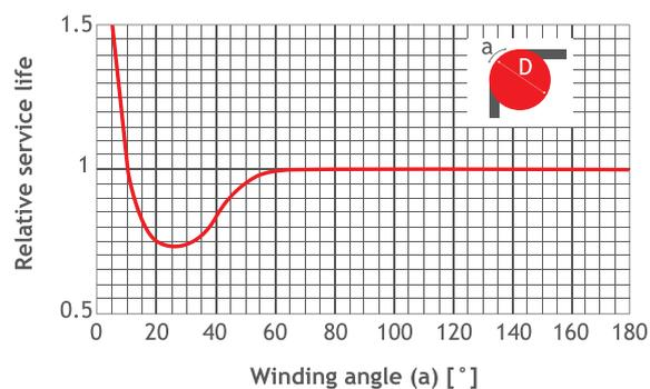
Figure 45 Relative service life depending on winding angle
