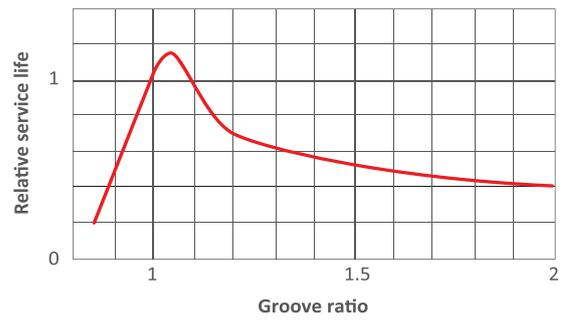
Figure 54 Effect of groove ratio on service life
