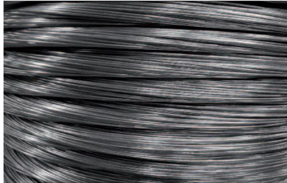
Figure 8 Galvanized wire
