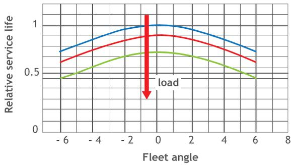
Figure 53 Effect of fleet angle on service life
