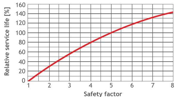
Figure 50 Effect of safety factor on service life
