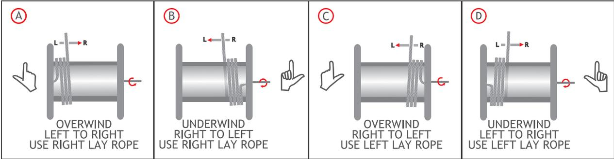
Figure 6 Selection of lay direction
