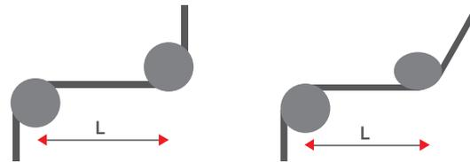
Figure 43 Reverse bending and partial reverse bending
